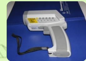
Infrared Temperature Measure
