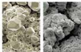
(Left) Microphotograph of a battery plate covered in heavy sulfation buildup (lead sulfate crystals).
