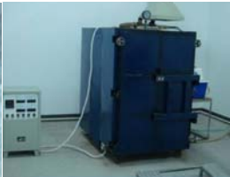
② Low-temperature thermal shock to remove the polarizing film
