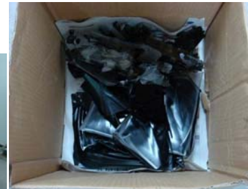
② Low-temperature thermal shock to remove the polarizing film
