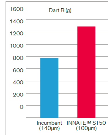
Mechanical properties for 100 \mu PE film for seed packaging against 140 \mu incumbent film
